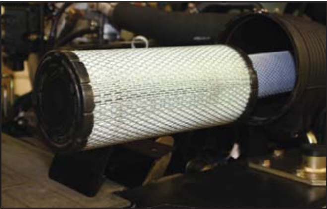
Dual element filters make doubly sure the air supplied is purified.
