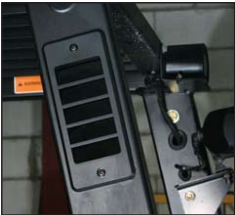
High air inlet in the overhead guard supplies cool and clean air to the engine.
